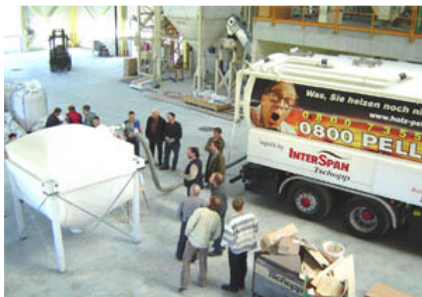
Füllung Sacksilo 3.2t in 7min
