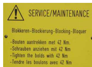
Fig. 13 Shield screw tightening torque
