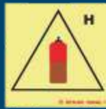
80.092 Remote release station of gas
