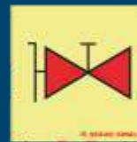
80.107 Fire main with fire valves
