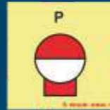
80.177 Fixed fire extinguisher powder bottle placed in a protected area
