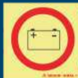
80.193 Emergency source of electrical power (battery)
