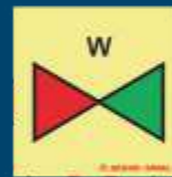
80.106 Fire main section valve
