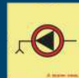
80.197 Emergency bilge pump
