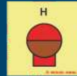
80.179 Fixed fire extinguisher gas bottle placed in a protected area
