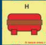
80.180 Fixed fire extinguisher gas installation
