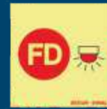
80.006 Space protected by automatic fire alarm
