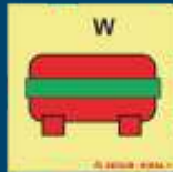
80.187 Fixed fire extinguisher water installation
