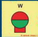
80.186 Fixed fire extinguisher water bottle placed in a protected area
