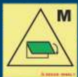
80.062 Remote control for closing devices of vent. inlet and outlet in machinery spaces
