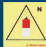
80.078 Remote release station of nitrogen
