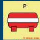
80.178 Fixed fire extinguisher powder installation
