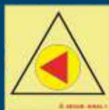
80.065 Fuel oil pump(s) remote shut-off
