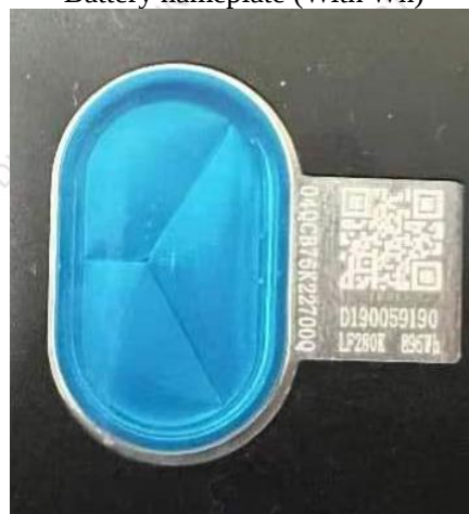
电池铭牌(含 Wh) Battery nameplate (With Wh)
