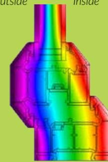
The cross section above shows how the multi-chambered profile prevents the transfer of heat from the inside to the outside.
