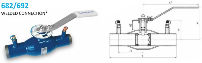
Temper balancing ball valves are designed for regulation (balancing) of the working fluid flow in heating, cold supply and ventilation systems. The ball has a special orifice and the valve is equipped with a scale of values. Regulation is carried out by turning the handle with the pointer. The selected position of the handle is fixed with a bolt and a nut-butterfly.
