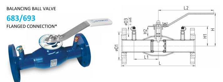
Temper balancing ball valves are designed for regulation (balancing) of the working fluid flow in heating, cold supply and ventilation systems. The ball has a special orifice and the valve is equipped with a scale of values. Regulation is carried out by turning the handle with the pointer. The selected position of the handle is fixed with a bolt and a nut-butterfly.
