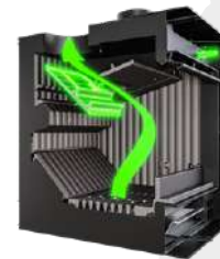
SMOKE BY-PASS ON
