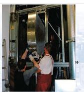
The replacement wheel is assembled in the housing of the old rotor. A new shaft, hub, and seals are included in the delivery.
