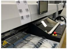
main steps: depositing the brazing paste, placing the components, soldering and automatic optical inspection. At the heart of the system, the placing machine, equipped with "Hydra" and "Mydas" heads, multiplies by a factor of three, the capacity for assembly while increasing the range of components available for TELERAD's products.
