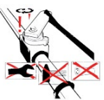
Don't operate a ball valve with a tool or an extension
