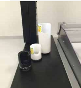
N.3 endoscopes supports for rigid and flexible endoscopes with closing cap for filling with disinfectant liquid.
