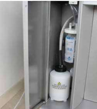
Surgical suction pump (dry pump) with 40 lt/min suction capacity. Ear-Washing funnel.
