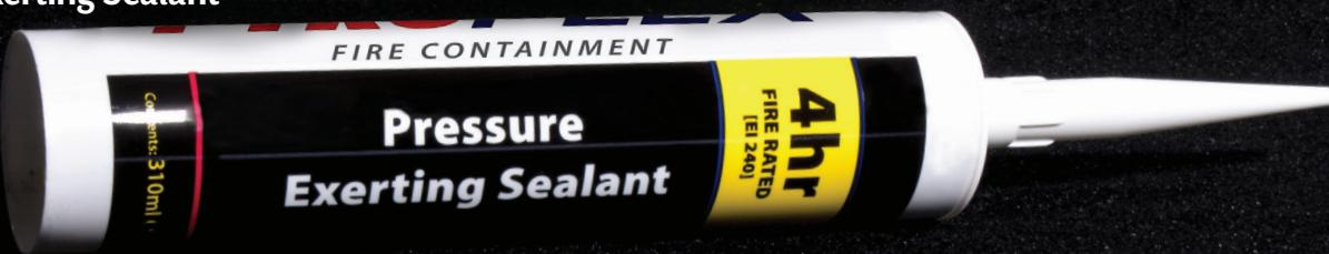
Pyroplex® Pressure Exerting Sealant expands multi-directionally when exposed to elevated temperatures, exerting pressure to seal and prevent the passage of fire and smoke through service penetrations. The sealant is designed for use around cable tray and bunched cable applications.
