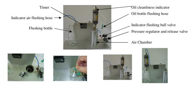
**EZ-LAB** is a stationary basis for testing oil cleanliness levels and oil viscosity from bottle oil samples, using **EZ-OilClean Check Indicator** and **EZ-Visco Check Indicator**.
