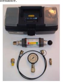
With EZ-OilClean Check you can test oil cleanliness levels any time, anywhere. On site tests will help you find out quickly the real condition of the oil and accomplish a better contamination control
