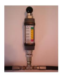
Particulate contamination of oil is the major source of wear and failure in hydraulic systems, bearings, gears and engines. It is very important to know the cleanliness level of your oil and make every effort to keep it clean. **EZ-OilClean Check** was specifically developed as a portable indicator for the maintenance staff to detect any fluid cleanliness changes, as a part of Proactive Maintenance.
